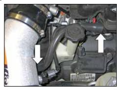
21. Attach the assembled vent hose onto the fitting installed in the K&N® intake tube; attach the open end of the vent hose to the valve cover port.
