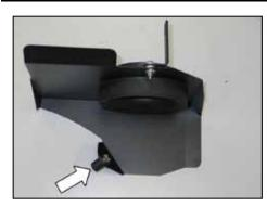
10. Install the provided rubber insert onto the heat shield as shown and secure with the provided hardware.
