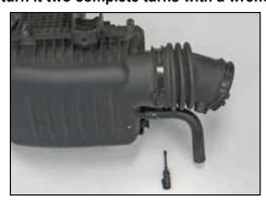
16. Remove the inlet air temperature sensor from the factory intake tube as shown.
