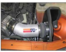
18. Install the K&N® intake tube into the silicone hump hose and then into the into the silicone step hose at the throttle body. Align the intake tube and heat shield for proper fit and then secure the intake tube with the provided hose clamps and heat shield bracket with the factory air box retaining bolt removed in an earlier step.
