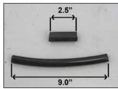
19. Cut the provided  $\frac{1}{2}$ " silicone vent hose to a length of 9" long. Also cut the  $\frac{5}{8}$ " vent line to a length of 2.5" long.
