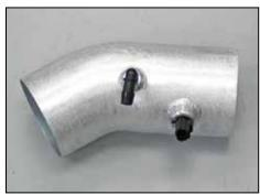
17. Install the inlet air temperature sensor into the  $K\&N^{\circ}$  intake tube as shown.
